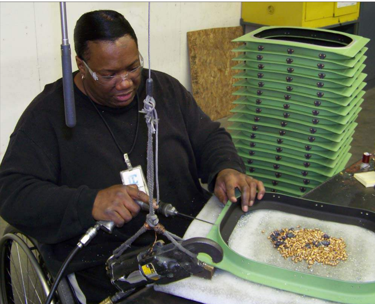
Damon Ross, Center Industries Corporation window frame assembler, installs nut plates on a Boeing 737 window frame for Spirit AeroSystems of Wichita, Kan. Center Industries Corporation has been the sole-source supplier of the 737 window frames for more than 20 years. Center is currently producing 4,000 frames per month and will continue to increase this quantity as the number of 737s being produced will ramp up from 31.5 per month to 35 by early 2012. (photo by Katie Link)
